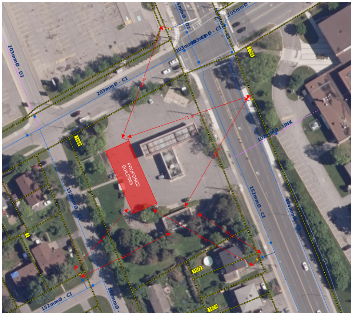
Figure 2 - Fire Hydrant Location
