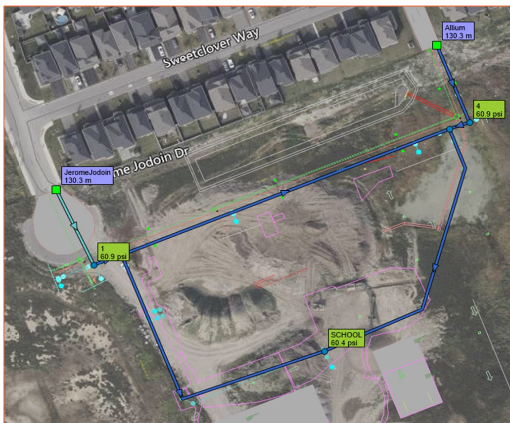
Figure 3.1: Maximum Pressures During AVDY Conditions
