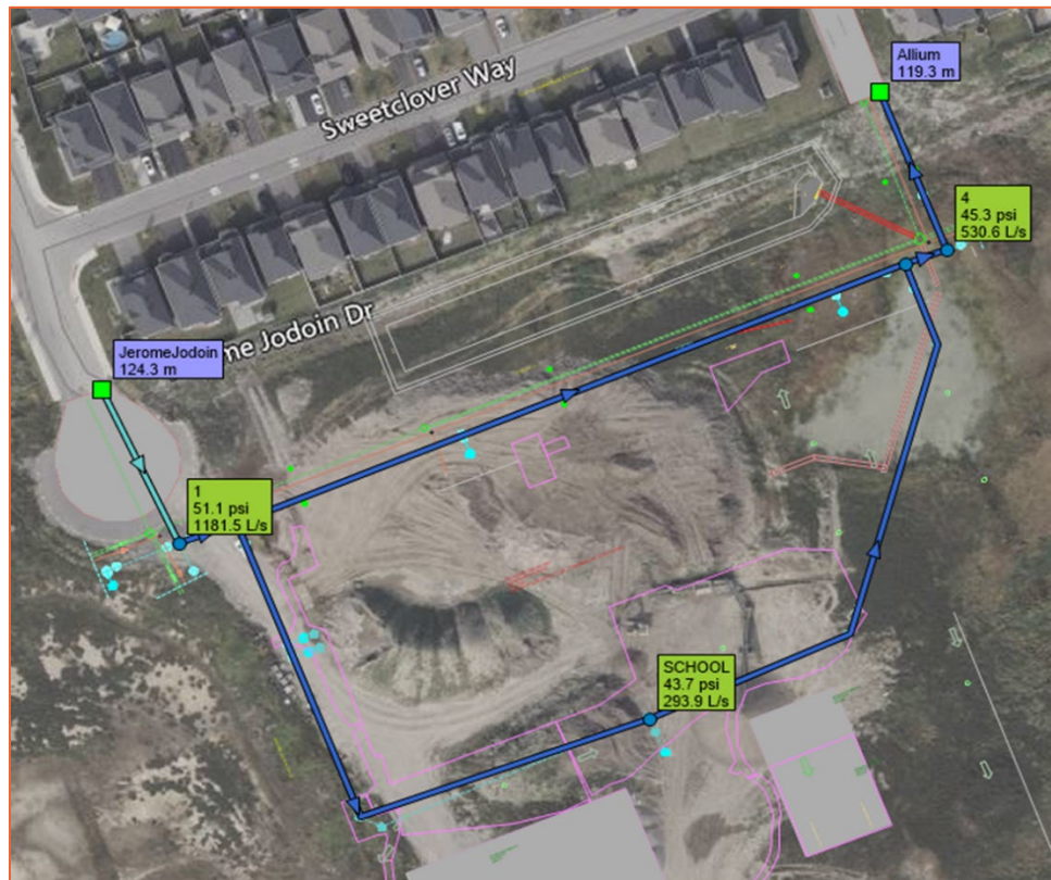
Figure 3.3: Residual Pressures and Available Fire Flows during MXDY Conditions (100 L/s)
