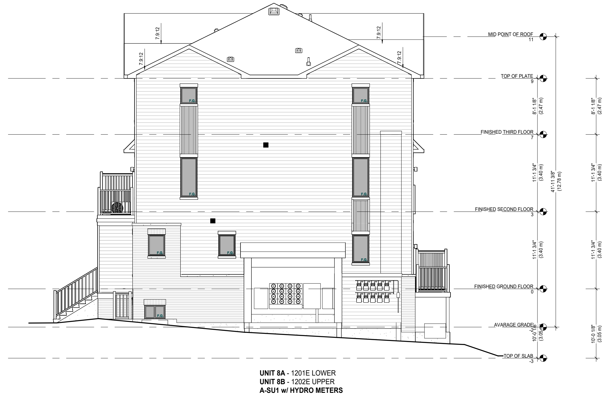
4 BLOCK 11 - UPGRADED RIGHT ELEVATION 'A' 1 : 96
