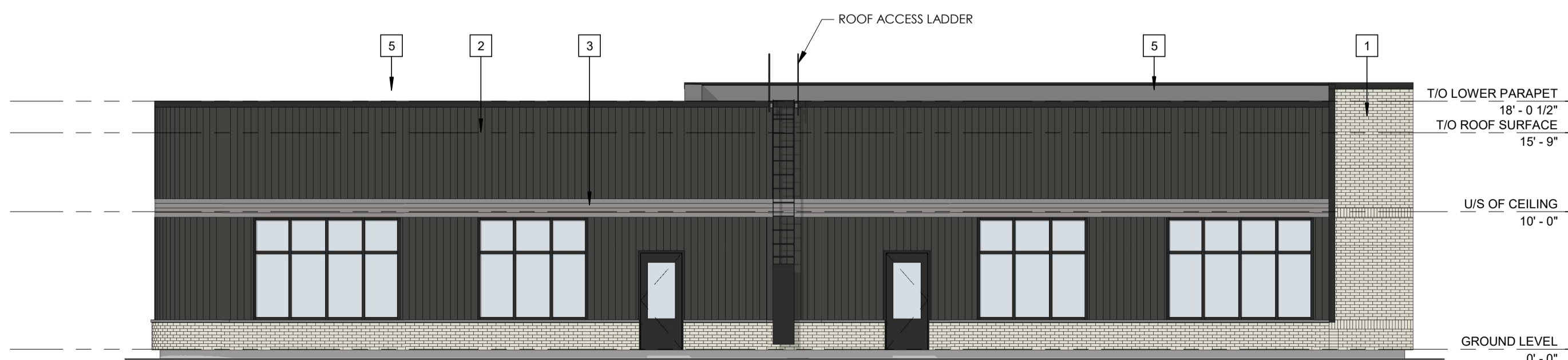
4 EAST DESIGN ELEVATION A4.00 1/8" = 1'-0" EXPOSING BUILDING FACE: 1,663 SF (154.5 m 2 ) GLAZING AREA: 279 SF (25.9 m 2 ) [16.8%] UNPROTECTED OPENING %: 16.8% LIMITING DISTANCE: 43'-11" (13.4 m)
