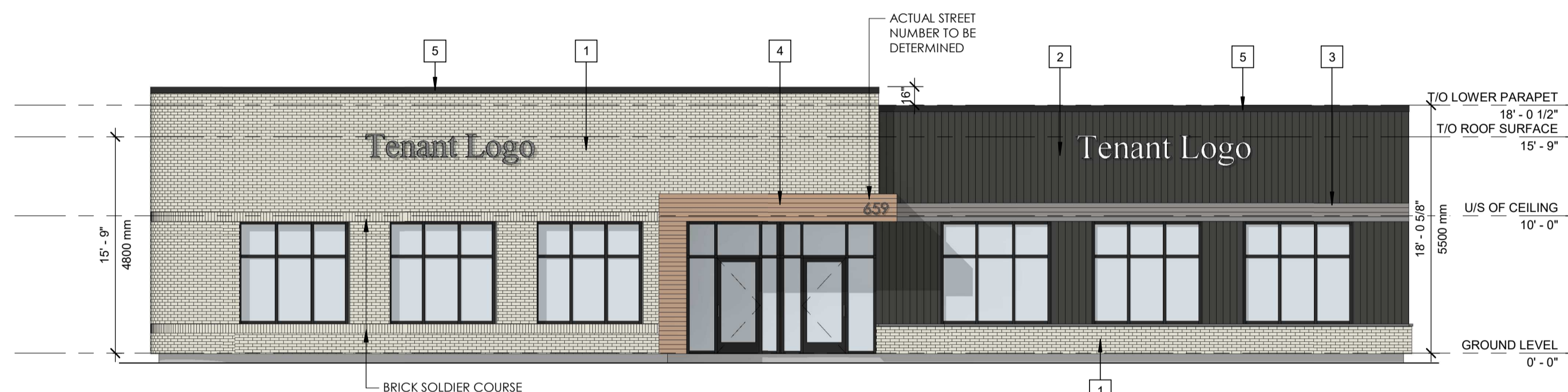
2 WEST DESIGN ELEVATION A4.00 1/8" = 1'-0" EXPOSING BUILDING FACE: 1,773 SF (164.7 m 2 ) GLAZING AREA: 479 SF (44.5 m 2 ) [27.0%] UNPROTECTED OPENING %: 27.0% LIMITING DISTANCE: 41'-4" 12.6 m
