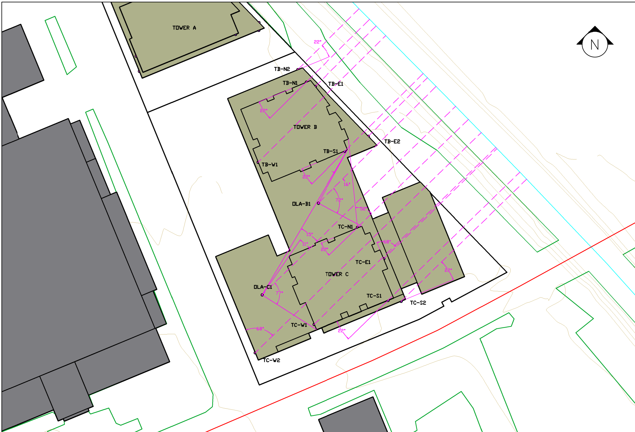
RECEPTOR EXPOSURE ANGLES FROM O-TRAIN TRILLIUM LINE - TOWERS B & C NOISE IMPACT STUDY ADDENDUM #2 - 145 LORETTA AVE N & 951 GLADSTONE AVE, OTTAWA
