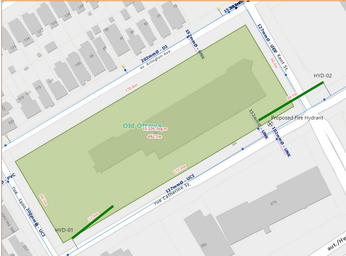
Figure 3.1: Fire Hydrant Coverage Sketch
