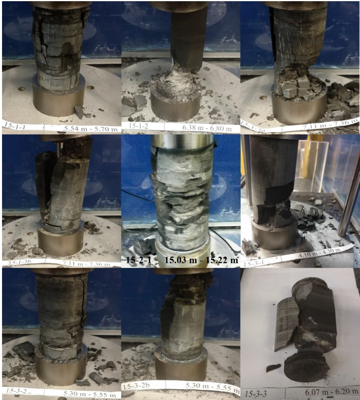
Figure 4: Photographs of UCS specimens after testing.
