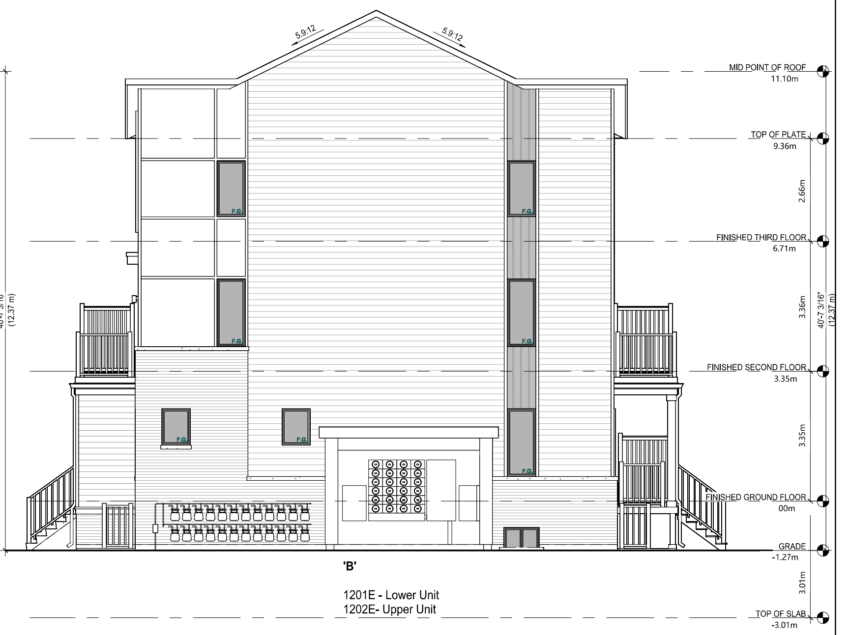
4 24 UNIT BLOCK - RIGHT ELEVATION 1:96
