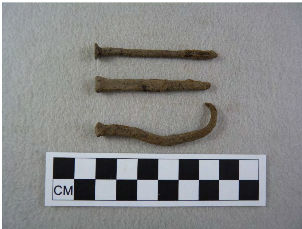
Image 41: (top) wire nail (28 S 0E), (middle) machine cut nail (28S 0E) and (bottom) wrought nail (30S 1W).
