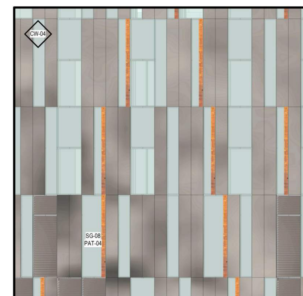
SPANDREL, VISION GLASS, PORCELAIN PANELS AND LOUVRES
