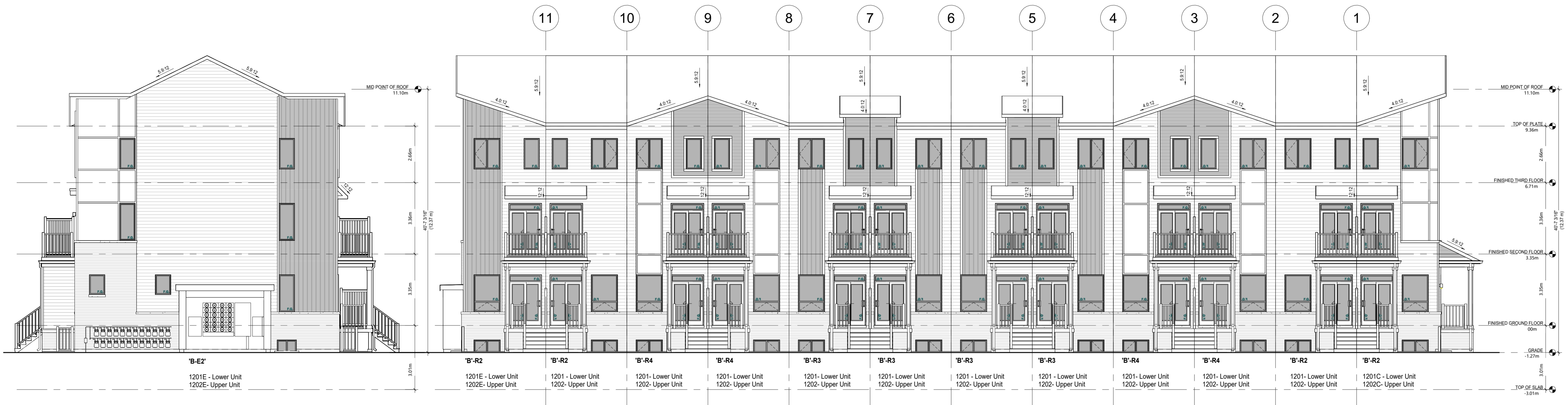
③ 24 UNIT BLOCK - UPGRADE RIGHT ELEVATION 1:96
