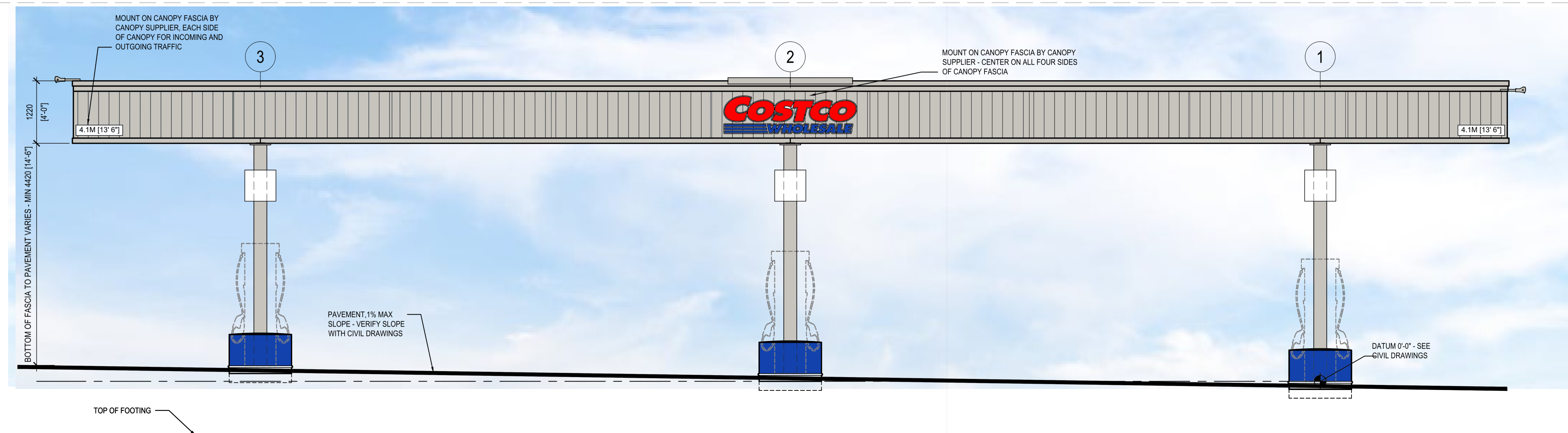
1 CANOPY AND DISPENSER ISLANDS (ENTRY ELEVATION)
