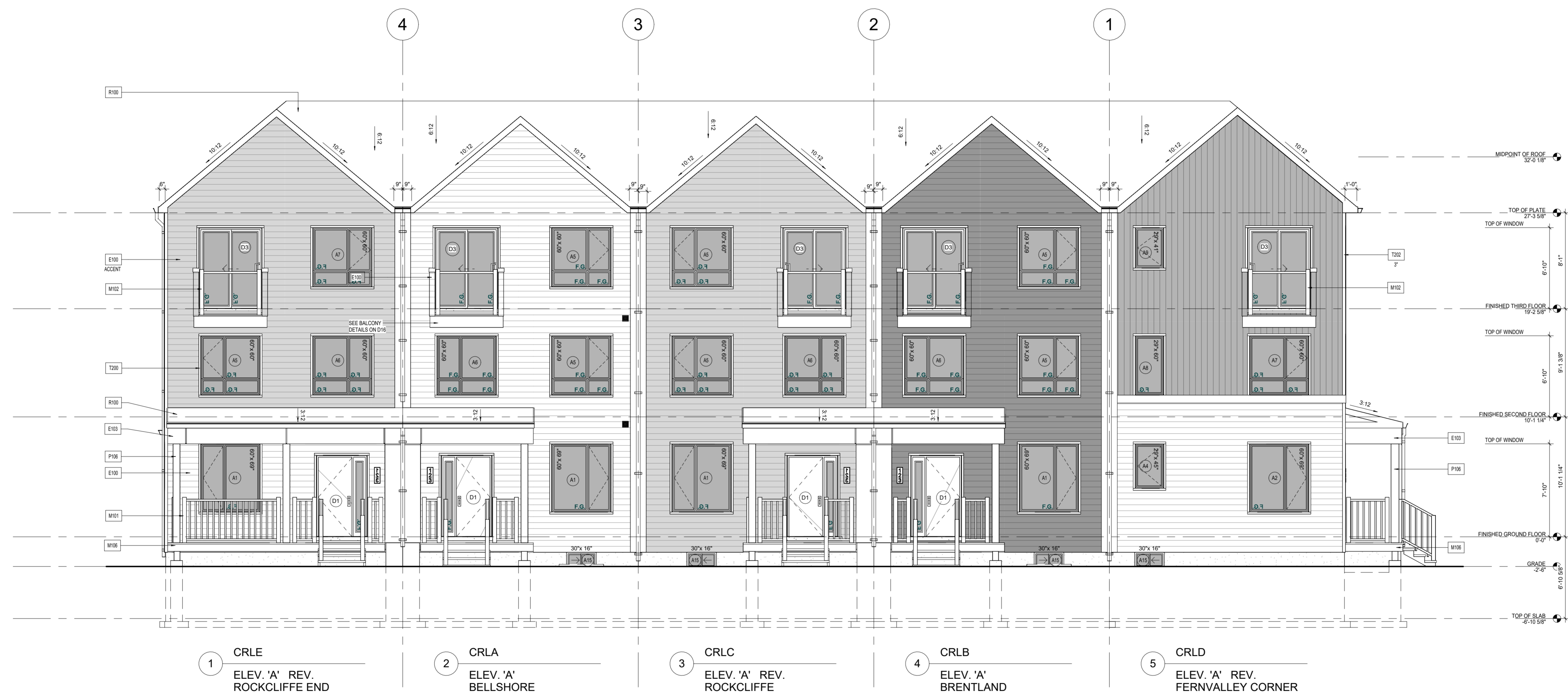
1 FRONT ELEVATION 'A' 3/16" = 1'-0"
