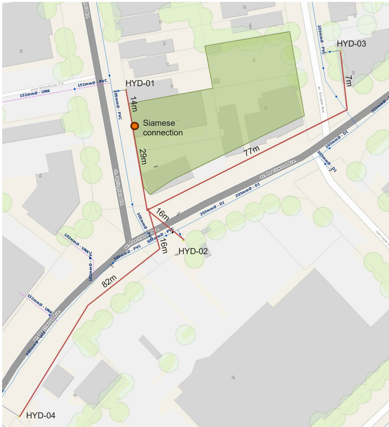
Figure 3-1: Fire Hydrant Coverage Sketch
