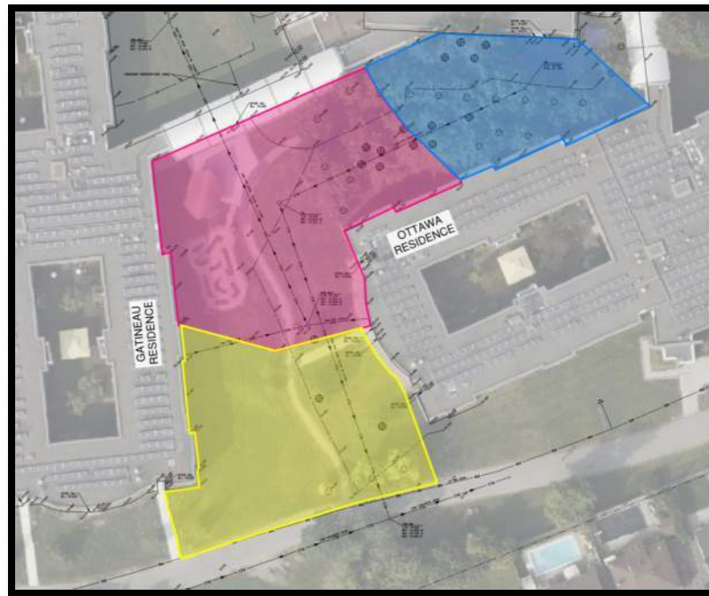
Figure 7: Existing Drainage Areas
