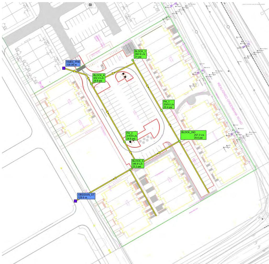
A fire flow of 15,000 L/min (250 L/s) was achieved at all serviced nodes. Sufficient fire flows for each block can be provided at every point within the distribution network for the proposed development.
