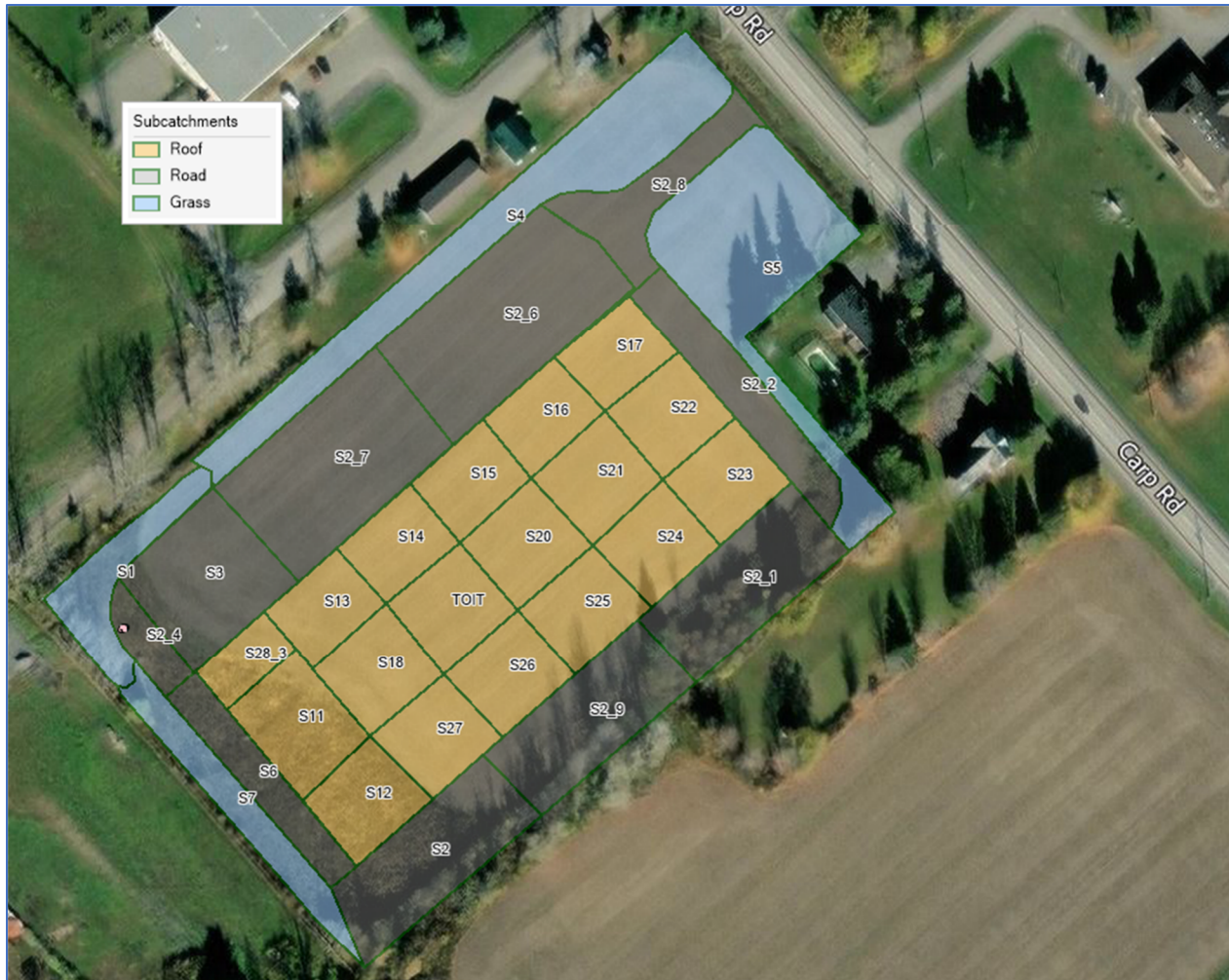
Figure 4: Stormwater Sub-catchments of the Study Site
