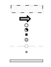
MAXIMUM STATIC PONDING LIMITS DIRECTION OF OVERLAND FLOW PROPOSED STORM SEWER PROPOSED CATCHBASIN MANHOLE PROPOSED CATCHBASIN CIRCULAR ORIFICE (SEE SEE ICD TABLE SD-1) EXISTING STORM SEWER
