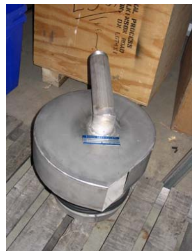
VHV with air vent for minimal slopes
