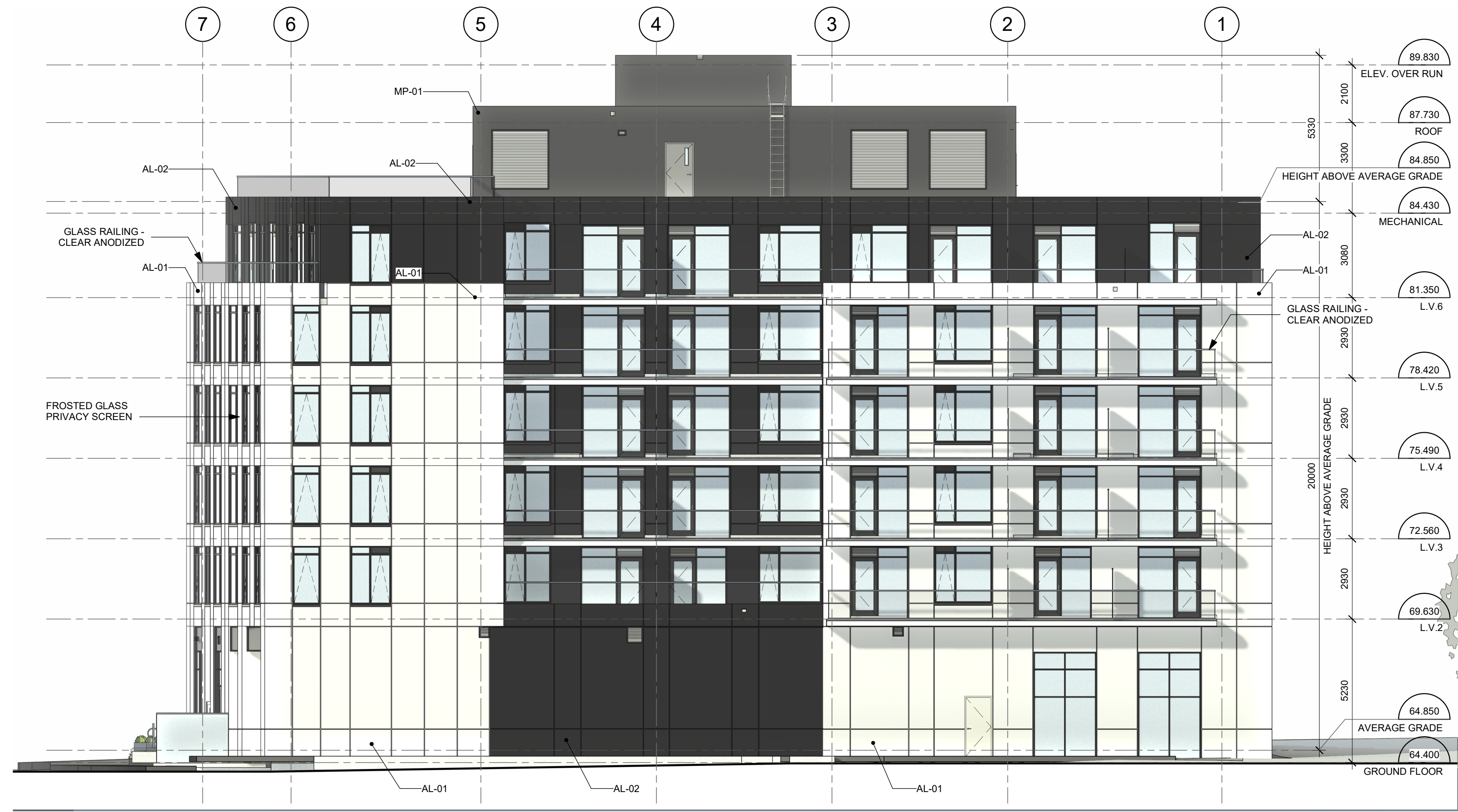
3 EAST ELEVATION D107 1:125
