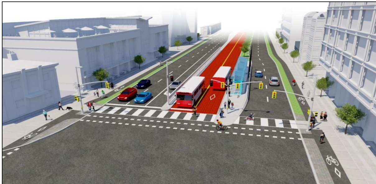
Figure 5: Median BRT lanes with station
