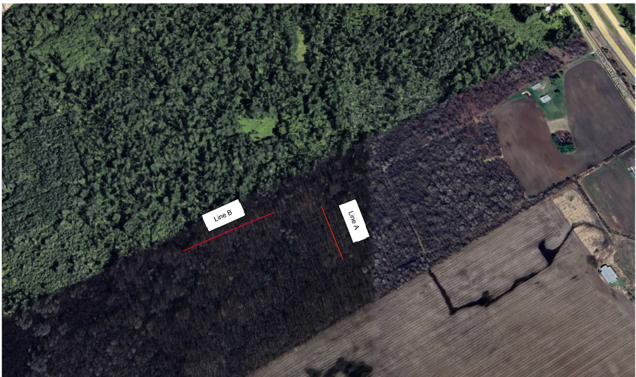
Figure 2: Site Map Showing VES Test Location (Red Line)
