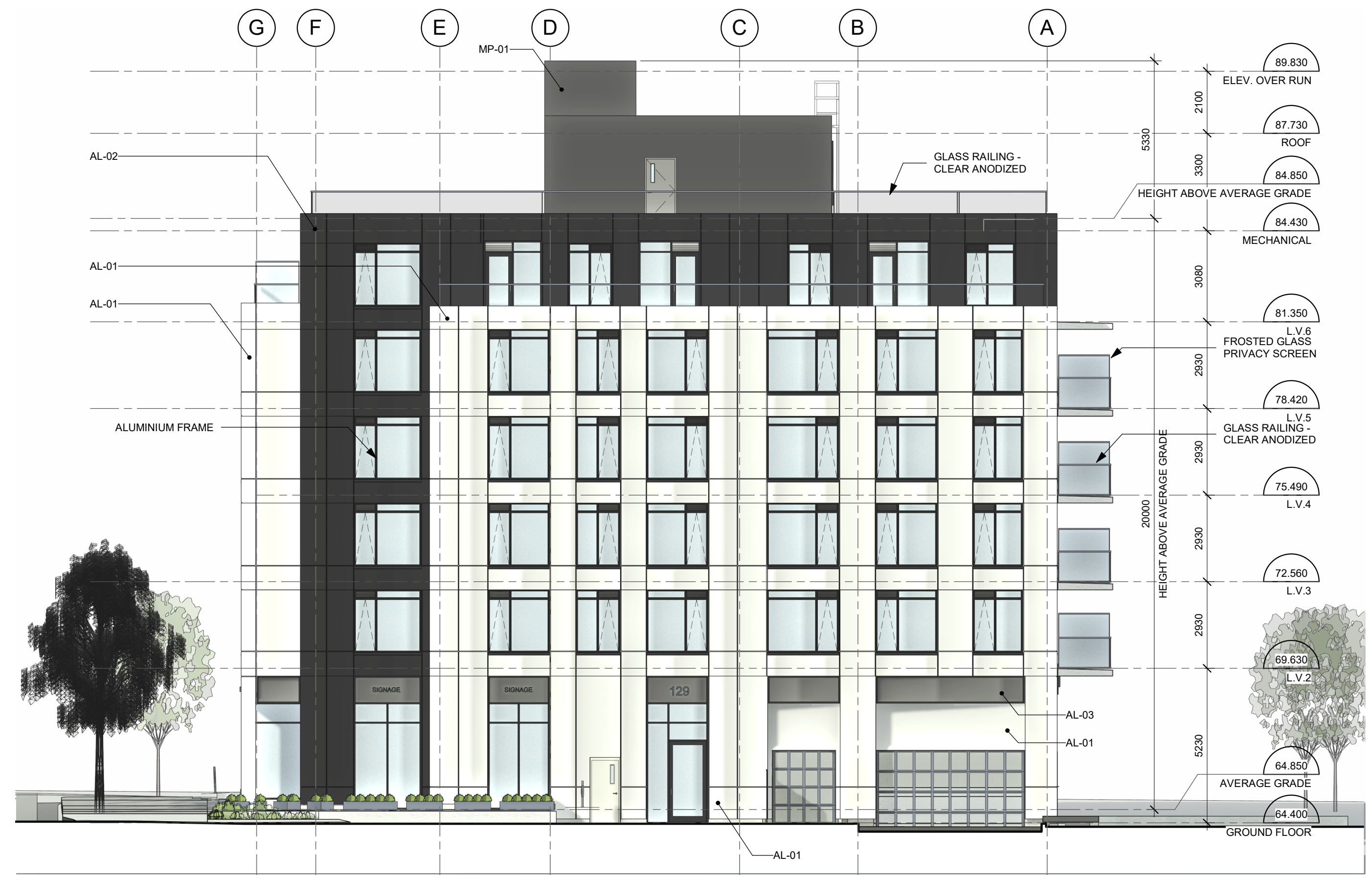
2 SOUTH ELEVATION - SPRINGHURST AVE D107 1 : 125
