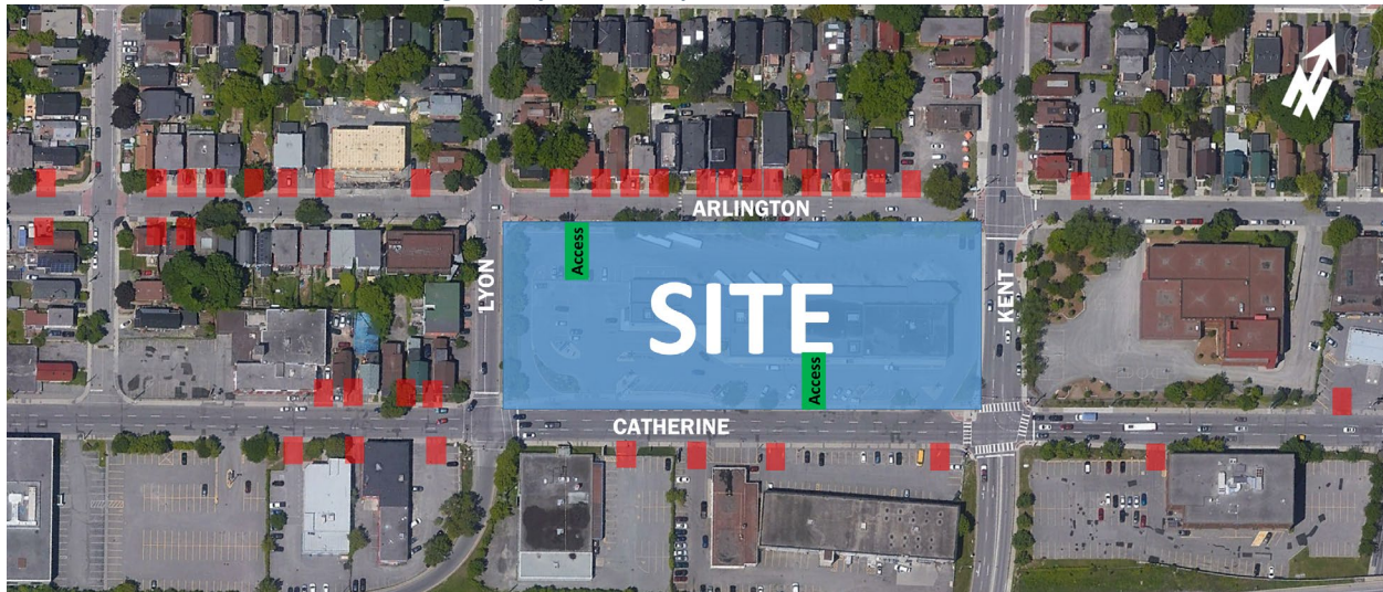
Figure 4: Adjacent Driveways within 200m of Site Access
