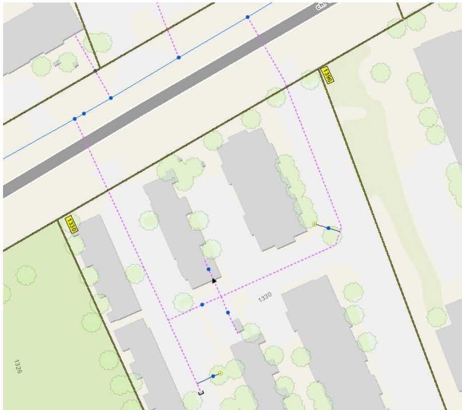
Figure 2: GeoOttawa Existing Water Services
