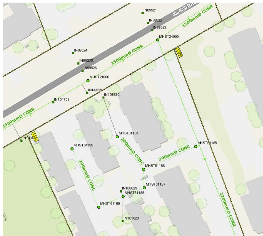
Figure 4: GeoOttawa Existing Storm Services
