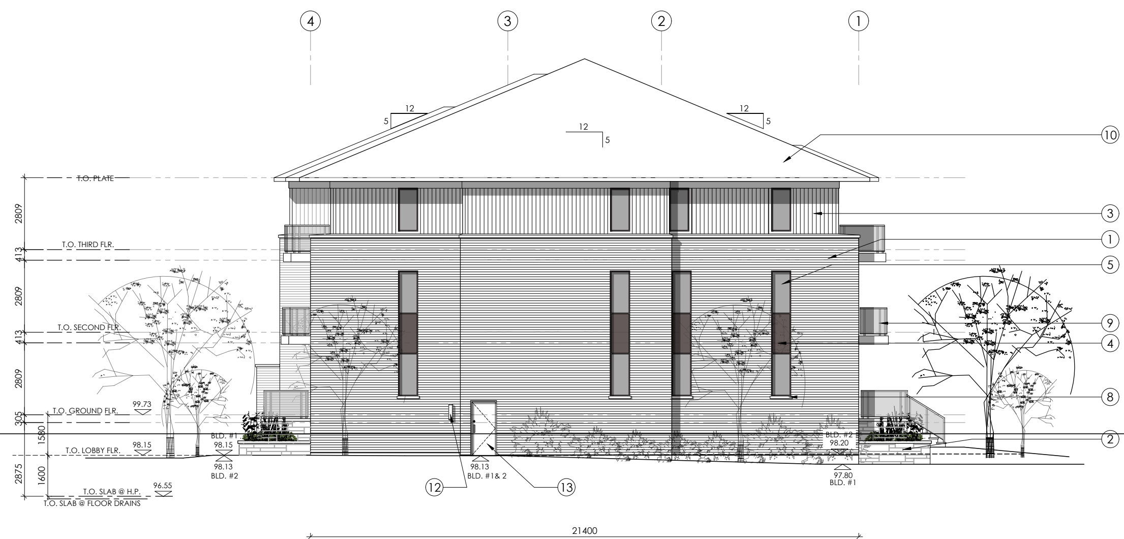
EXTERIOR SIDE (SOUTH or NORTH) ELEVATION SCALE= 1:150 (BUILDING #1 NORTH ELEVATION SHOWN) (BUILDING #2 SOUTH ELEVATION SHOWN IN REVERSE)
