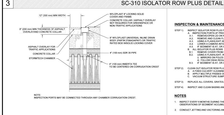
4" PVC INSPECTION PORT DETAIL (SC SERIES CHAMBER)
