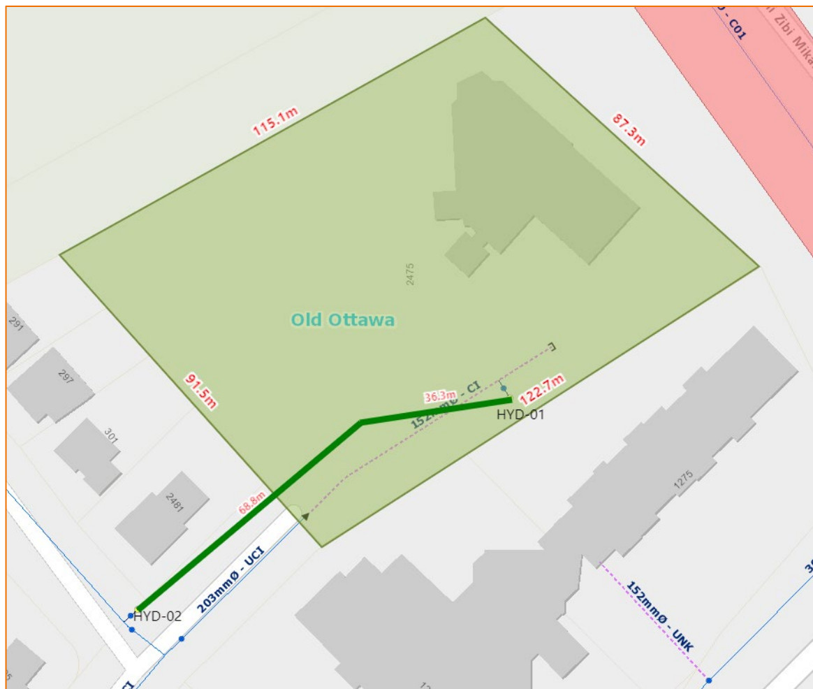
Figure 3.1: Existing Fire Hydrant Coverage Map
