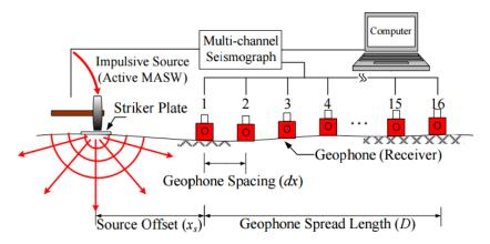
Figure 1 Schematic Layout of MASW Test Setup (Sahadewa et al., 2012<sup>2</sup>)
