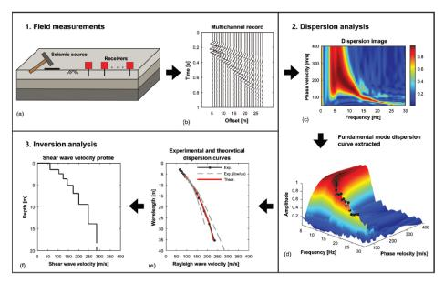
Figure 2 Overview of MASW method (Olafsdottir et al., 2018<sup>3</sup>)
