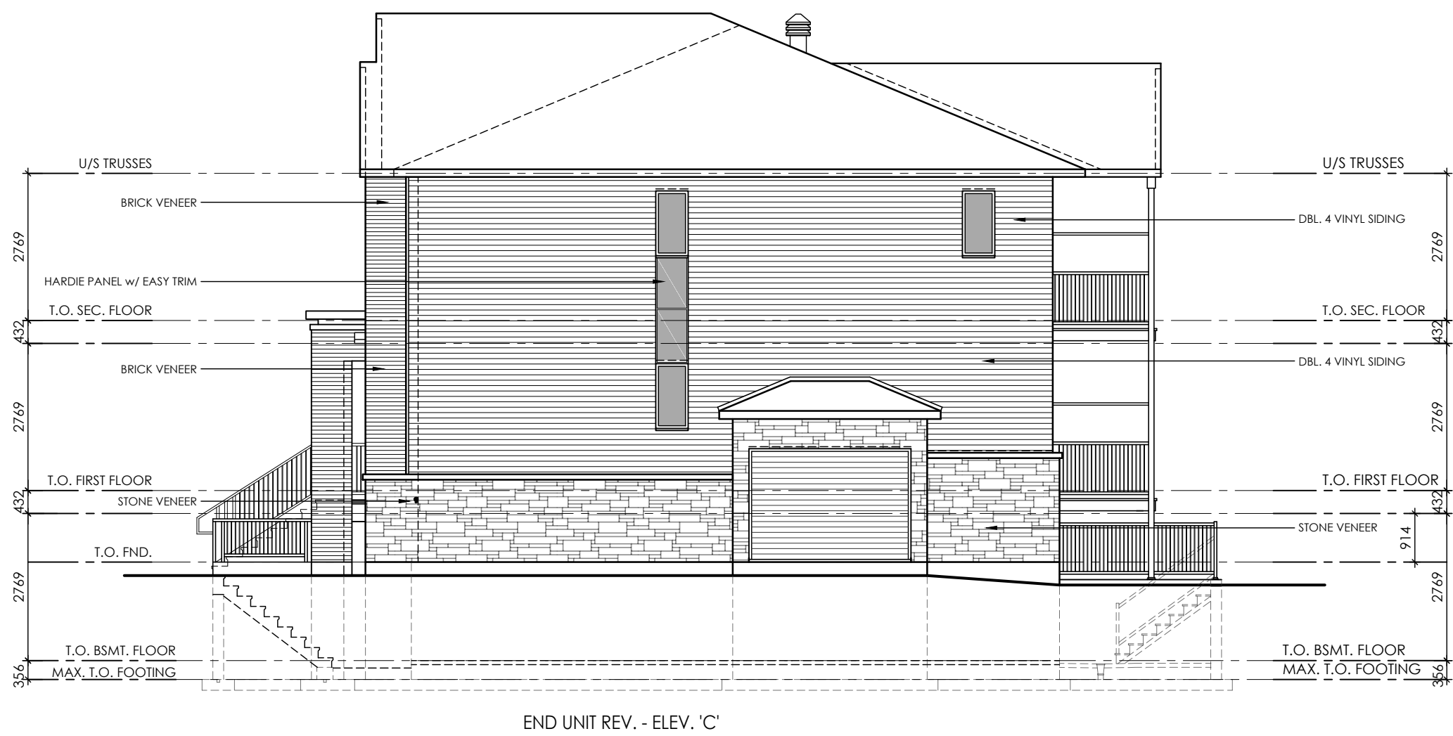
TYPICAL BLOCK - INTERIOR SIDE ELEVATION
