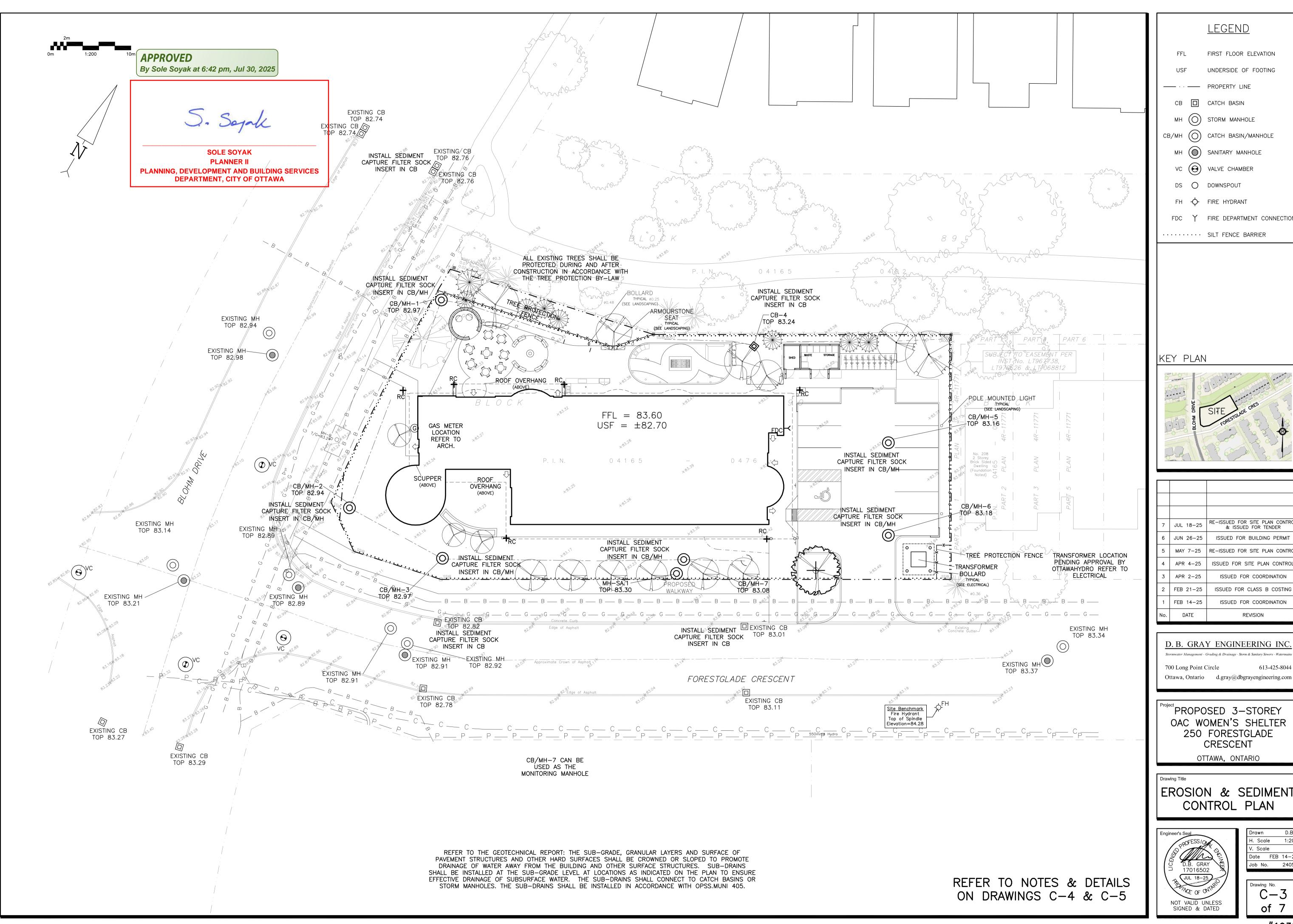
**LEGEND** FIRST FLOOR ELEVATION UNDERSIDE OF FOOTING CATCH BASIN () STORM MANHOLE CB/MH (O) CATCH BASIN/MANHOLE ( SANITARY MANHOLE VALVE CHAMBER DS O DOWNSPOUT -O- FIRE HYDRANT FDC Y FIRE DEPARTMENT CONNECTION · · · · · · · · · SILT FENCE BARRIER
