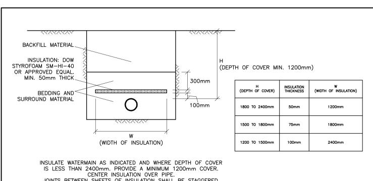
JOINTS BETWEEN SHEETS OF INSULATION SHALL BE STAGGERED. INSULATION OF WATERMAINS & WATER SERVICE CONNECTIONS IN SHALLOW TRENCHES N.T.S
