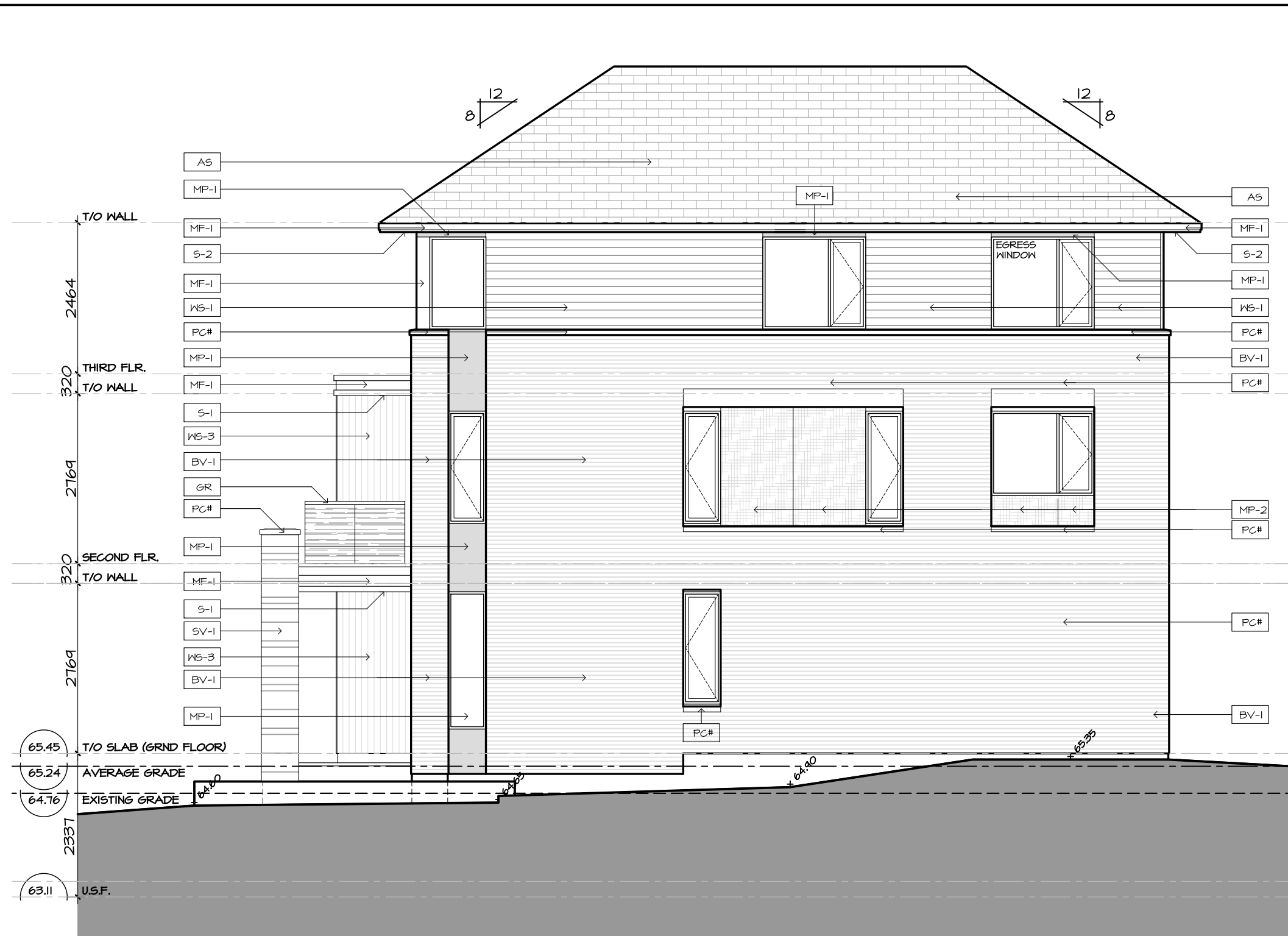
2 | BLOCK T1 - NORTH ELEVATION
