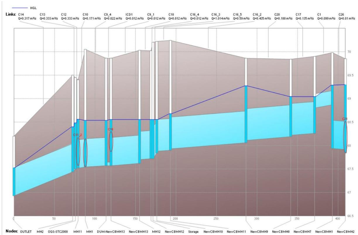
**Figure 5.10. Proposed Conditions Hydraulic Grade Line Profile for the Storm Sewer around the ZEB Garage for the 100-Year Storm Event**
