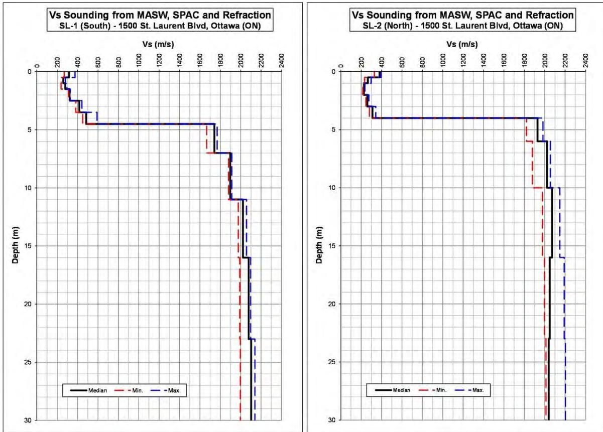
**Figure 5: MASW Shear-Wave Velocity Soundings**
