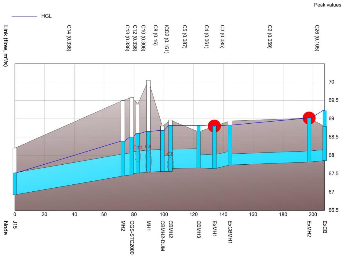
**Figure 5.6. Existing Hydraulic Grade Line Profile for the Sewer Parallel to the North Garage for the 100-Year Storm Event**
