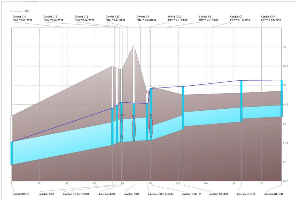
**Figure 5.12. Proposed Conditions Hydraulic Grade Line Profile for the Sewer North of the North Garage for the 100-Year Storm Event**
