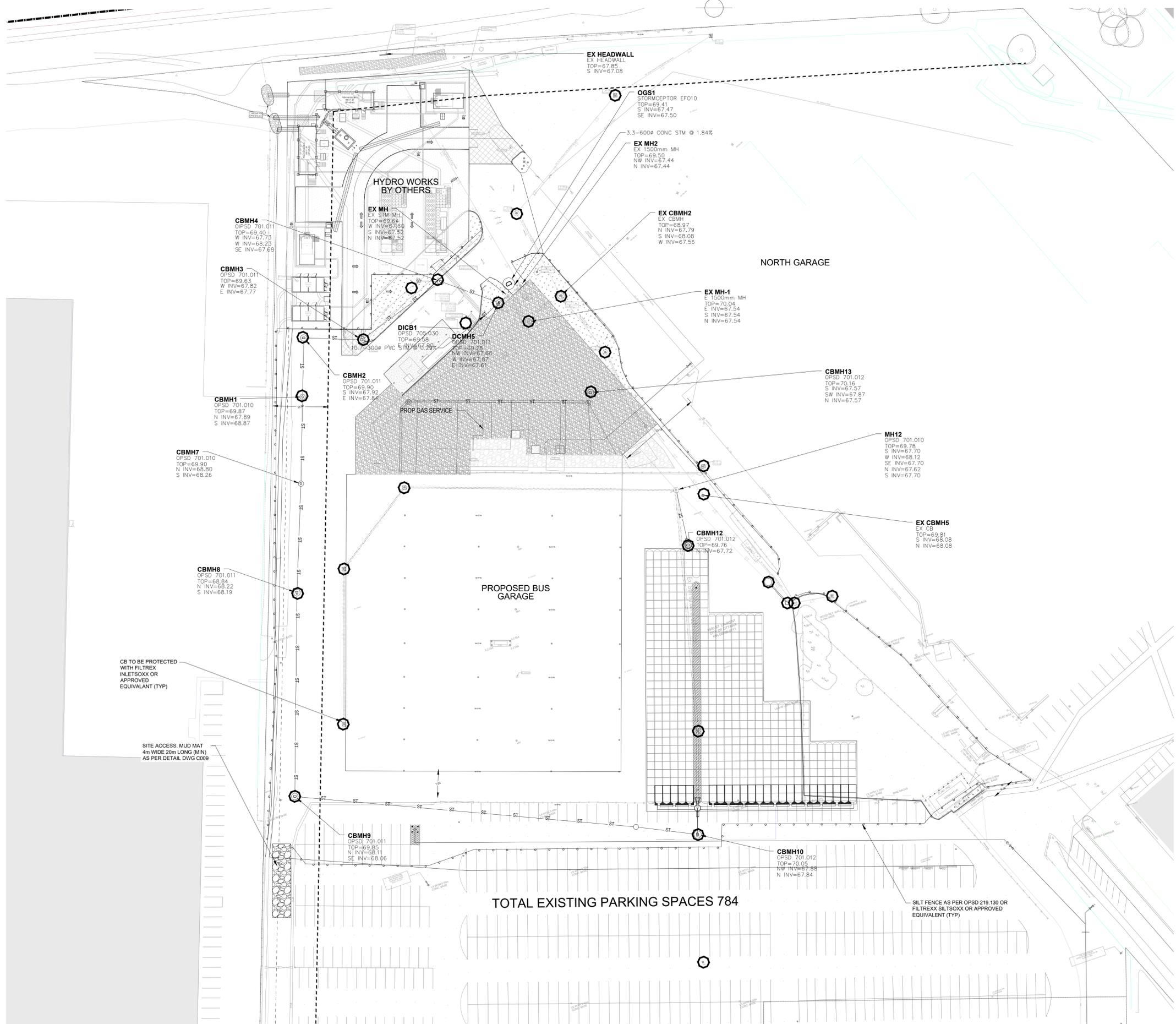
CB TO BE PROTECTED WITH FILTREX INLETS/XX OR APPROVED EQUIVALENT (TYP)
