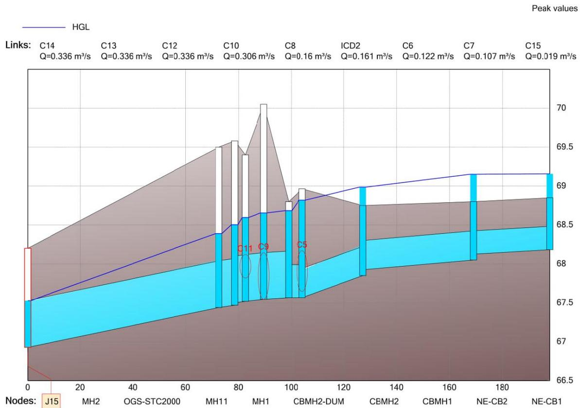
**Figure 5.7. Existing Hydraulic Grade Line Profile for the Sewer North of the North Garage for the 100-Year Storm Event**
