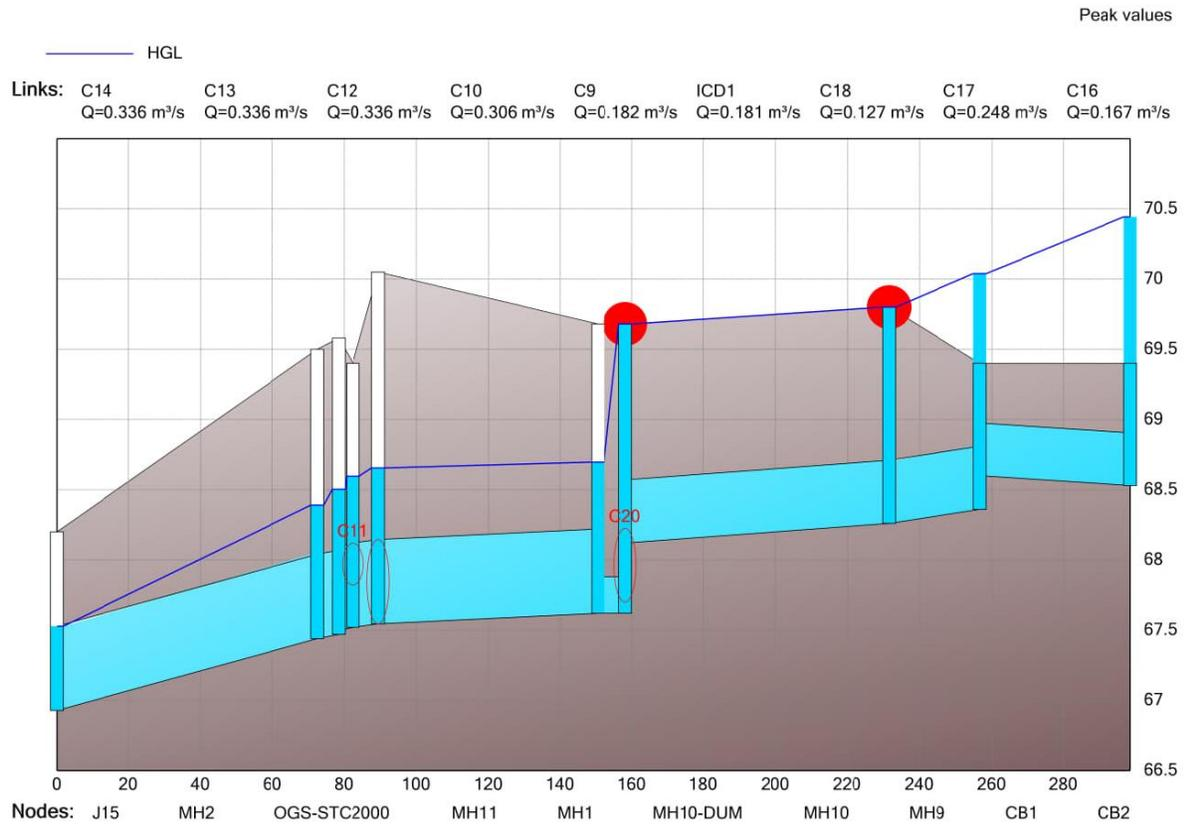
**Figure 5.5. Existing Hydraulic Grade Line Profile for the Bus Parking Lot Storm Sewer for the 100-Year Storm Event**
