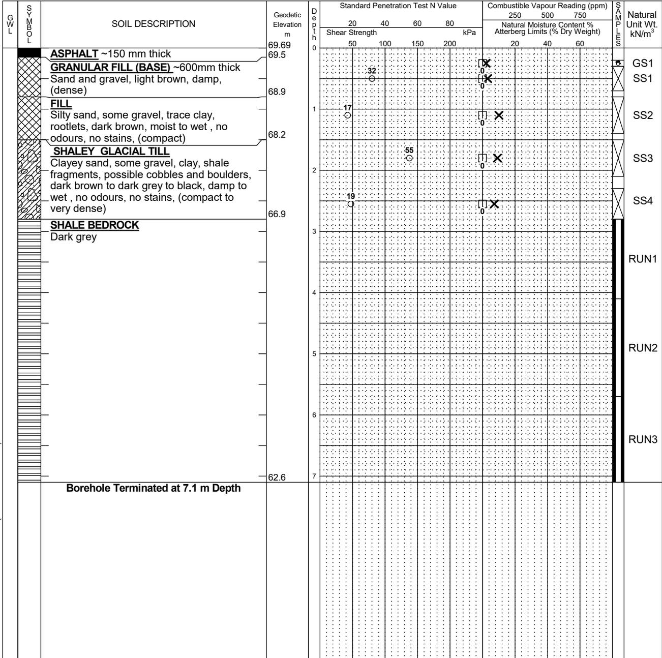
LOG OF BOREHOLE OTT-22007382 - 1500 SAINT LAURENT BH LOGS (NEW BUS GARAGE) GPJ TROW OTTAWA.GDT 06/12/24
