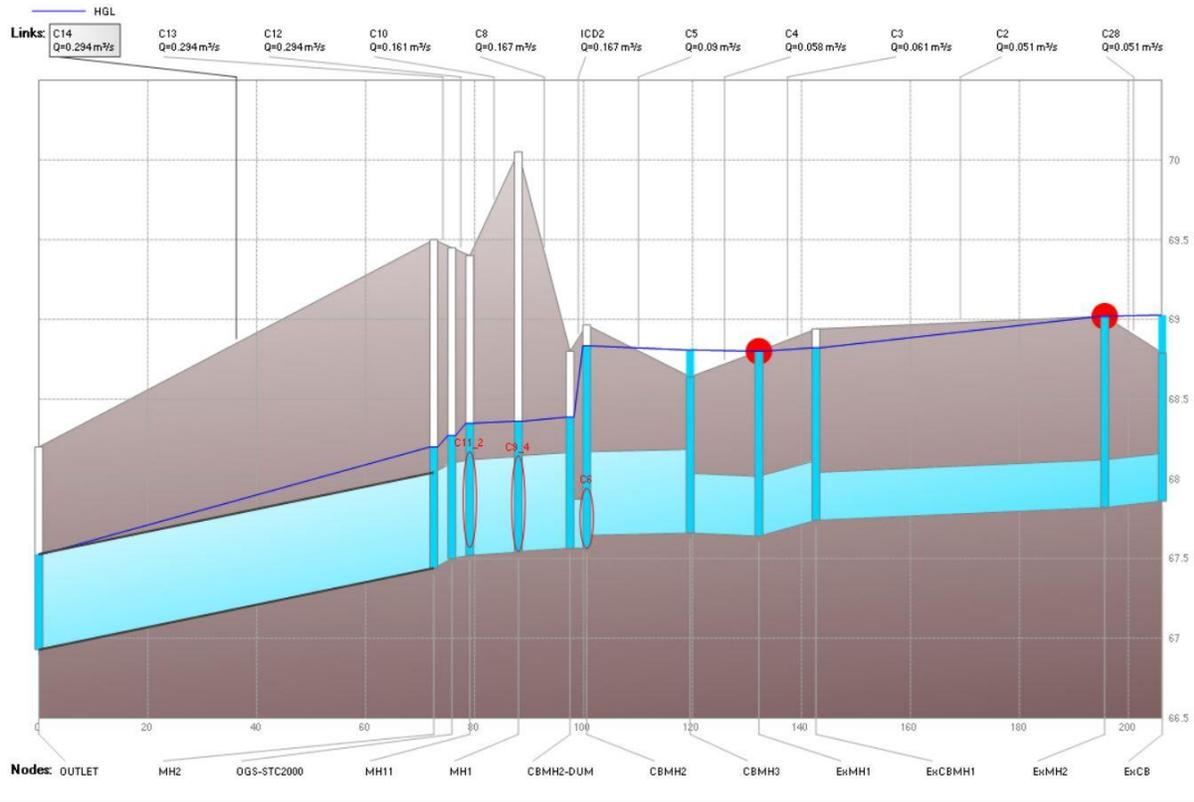
**Figure 5.11. Proposed Conditions Hydraulic Grade Line Profile for the Sewer Parallel to the North Garage for the 100-Year Storm Event**
