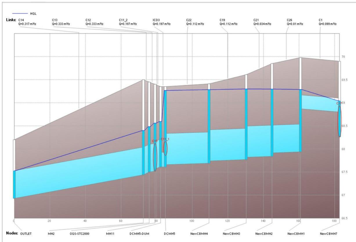
**Figure 5.13. Proposed Conditions Hydraulic Grade Line Profile for the Sewer South of the Substation for the 100-Year Storm Event**
