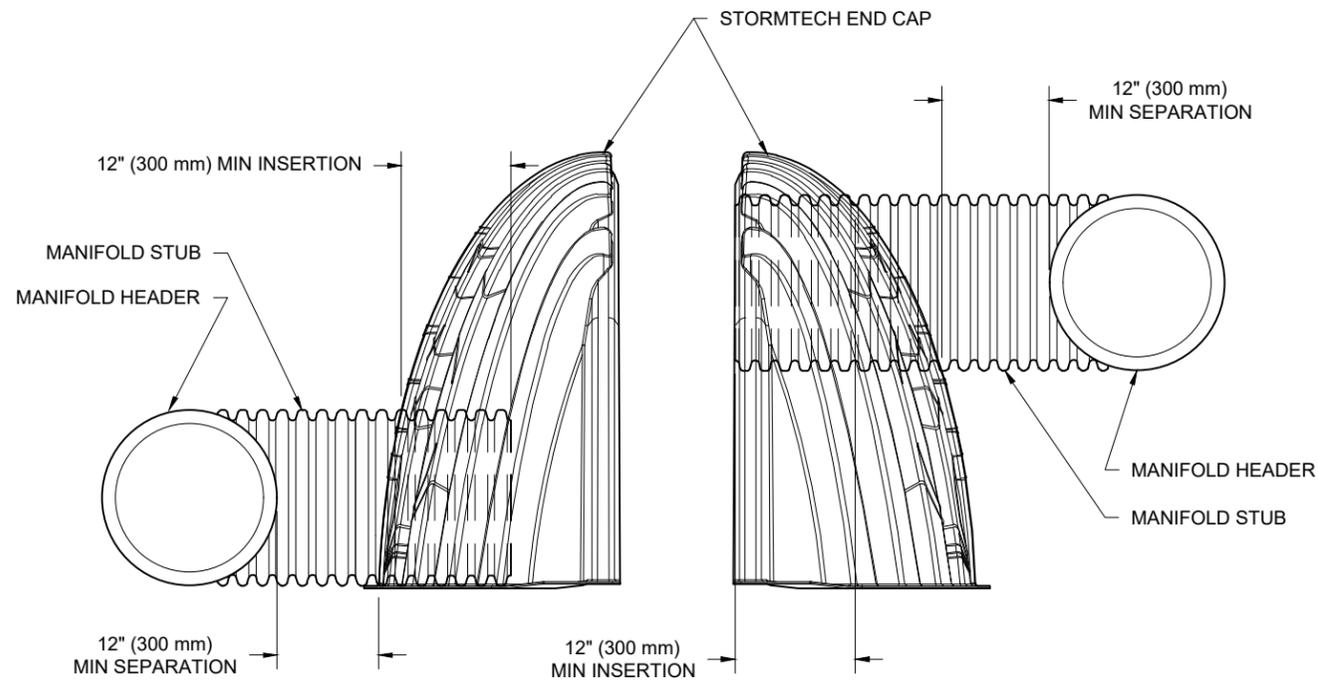
NOTE: MANIFOLD STUB MUST BE LAID HORIZONTAL FOR A PROPER FIT IN END CAP OPENING.
