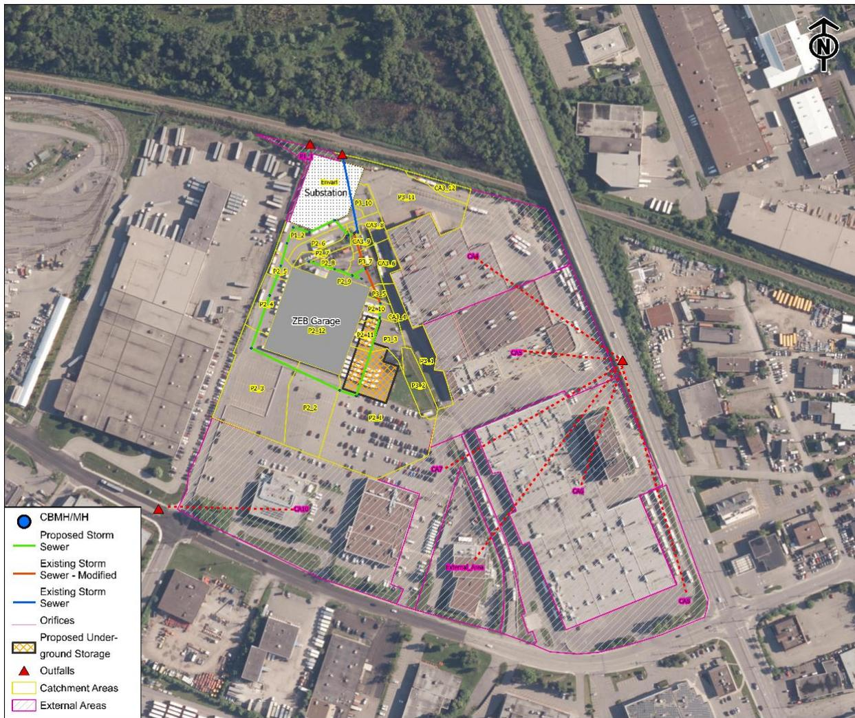
**Figure 5.8. Proposed Conditions Catchment Area and Storm Sewer for the Northwest Corner as Represented in PCSWMM**
