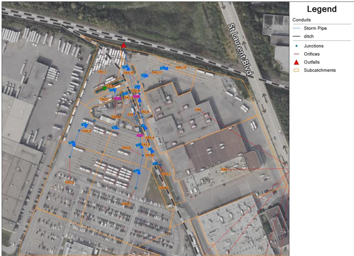
**Figure 5.4. Existing Conditions Catchment Area and Storm Sewer for the Northwest Corner as Represented in PCSWMM**
