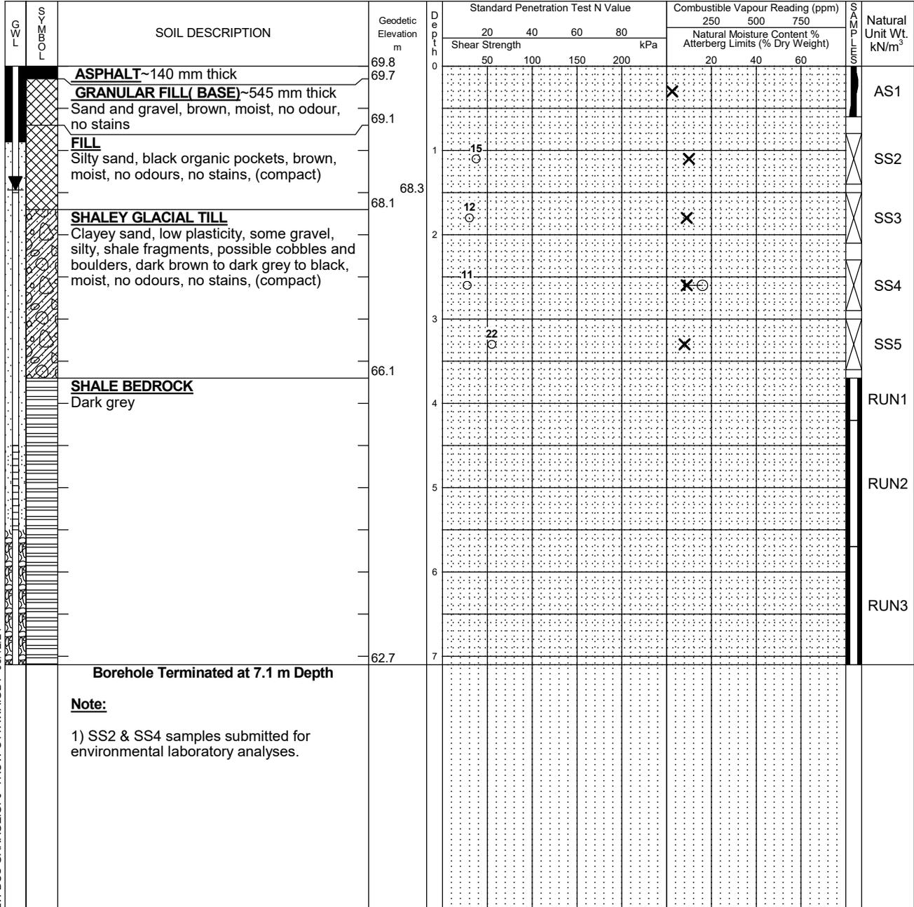
LOG OF BOREHOLE BH LOGS-NEW BUS GARAGE.GPJ TROW OTTAWA.GDT 06/12/24
