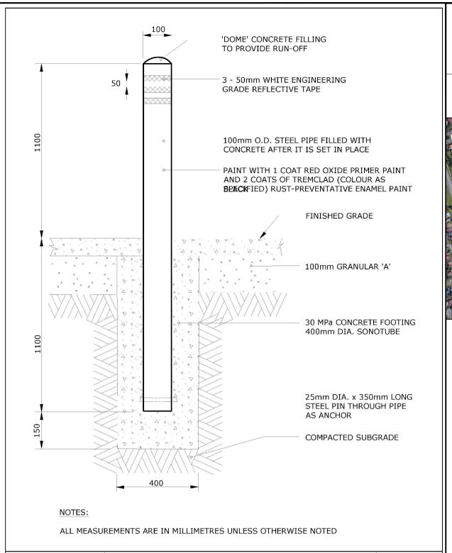
100mm DIAMETER STEEL BOLLARD
