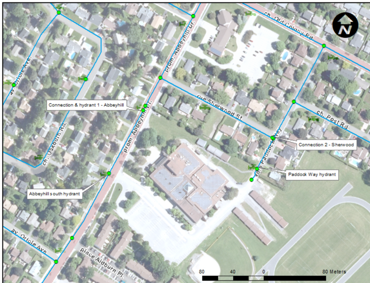
Figure 1: Existing hydrant configuration & connections
