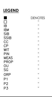
FOUND MONUMENTS SEI MONUMENIS IRON BAR ROUND IRON BAR STANDARD IRON BAR SHORT STANDARD IRON BAR CUT CROSS CONCRETE PIN WITNESS PROPERTY IDENTIFICATION NUMBER MEASURED PROPORTIONED ORIGIN UNKNOWN STANTEC GEOMATICS LTD. OBSERVED REFERENCE POINT PLAN 4R-32043 PLAN 4R-26139 PLAN 4R-36547
