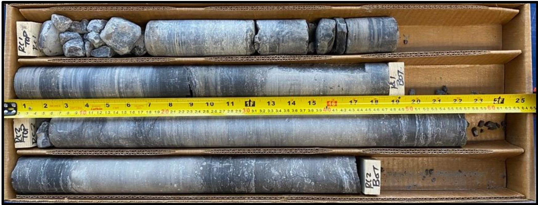
Photograph of Rock Core obtained from BH 2-25 from interval RC1 and RC2
