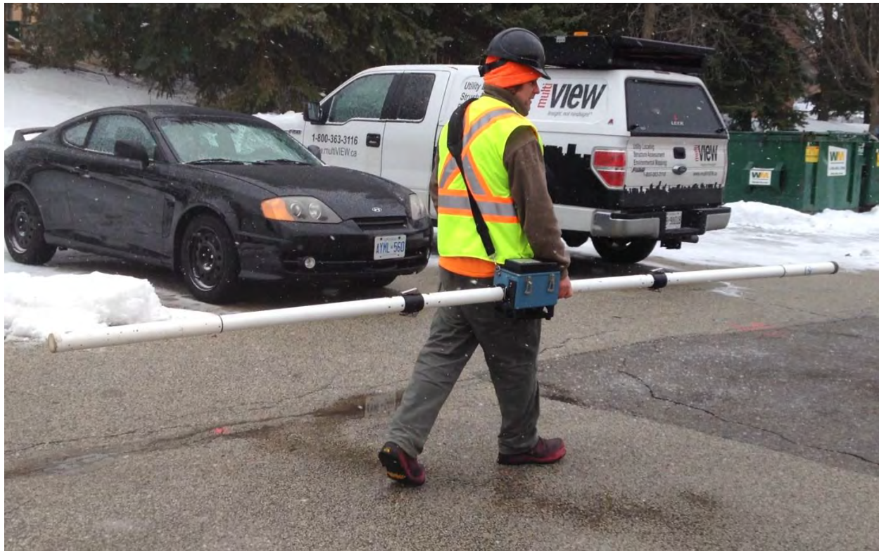
Figure 3-2: Typical FDEM Acquisition System Setup
