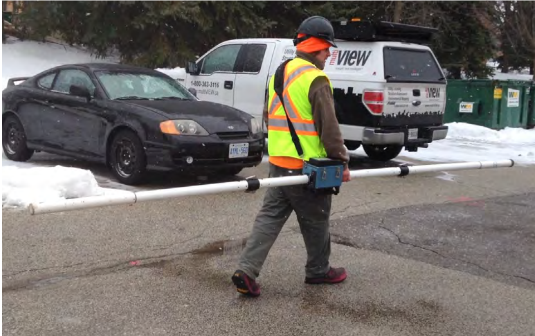
Figure 4: Photo Illustrating a Typical Frequency Domain EM31 Acquisition System Setup
