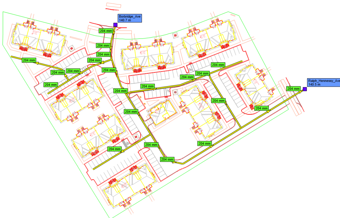
Figure 3.1 Proposed Watermain Layout and Pipe Diameters (mm)
