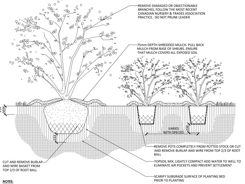
GRASSES 25mm HIGHER THAN ADJACENT GRADE -75mm SHREDDED MULCH, PULL BACK MULCH FROM BASE OF PLANT. ENSURE THAT MULCH COVERS ALL EXPOSED SOIL CONTRUCT 100mm SAUCER AROUND PERENNIAL / GRASS SCARIFY SUBGRADE SURFACE OF-TOPSOIL MIX, LIGHTLY COMPACT TO ELIMINATE AIR POCKETS PLANTING BED PRIOR TO AND PREVENT SETTLEMENT PLANTING REMOVE POTS COMPLETELY FROM POTTED STOCK OR CUT COMPACTED SUBGRADE— AND REMOVE BURLAP AND WIRE FROM TOP 2/3 OF ROOT
