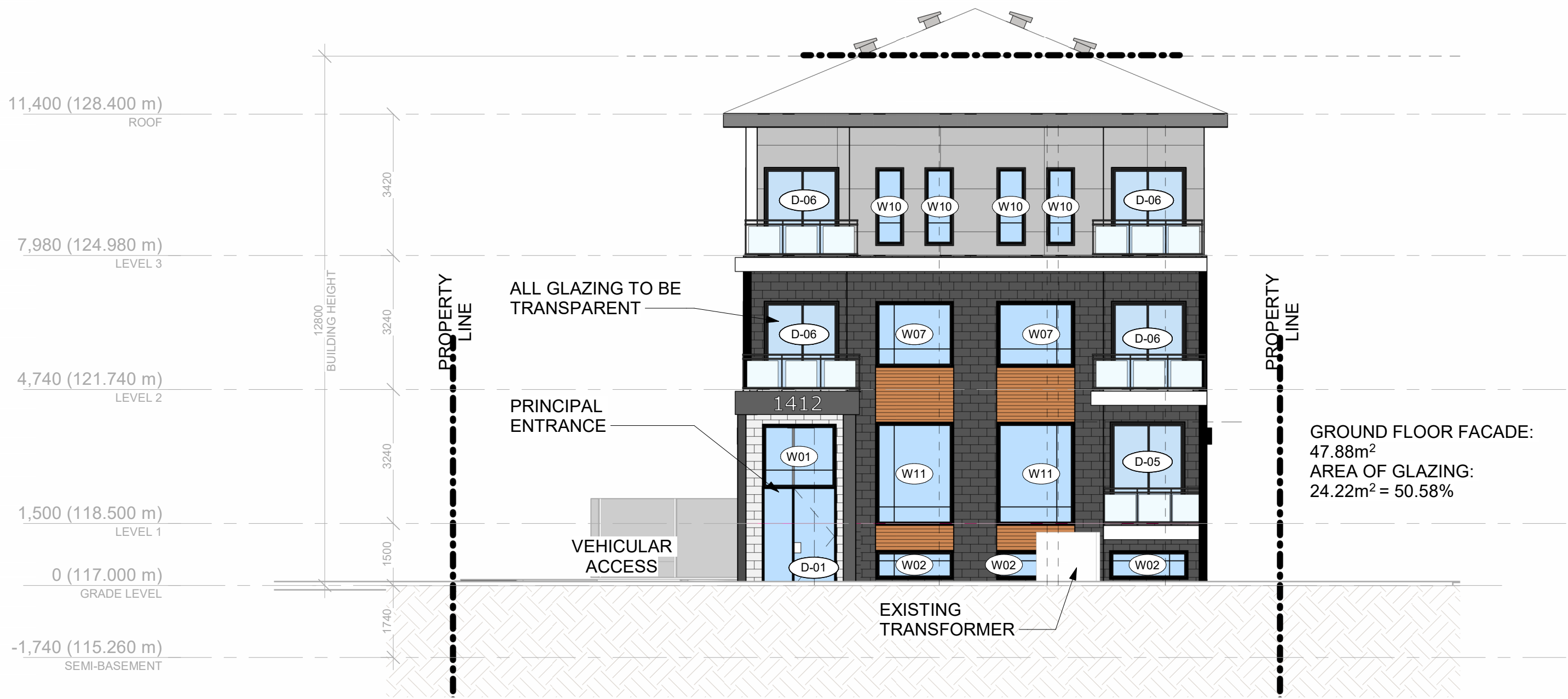
1 NORTHEAST ELEVATION - STITTSVILLE MAIN (FRONT) 1 : 100
