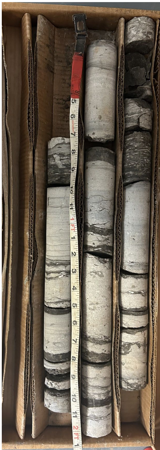
Photo 1: Rock Core Run 1 & 2, BH105-24, 39.0 to 41.8 mbgs
