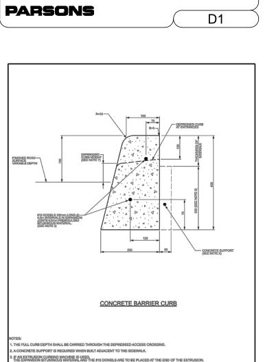
CONCRETE BARRIER CURB FOR GRANULAR BASE PAVEMENT
