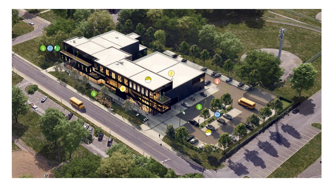
A geothermal system consisting of 15 wells provides the heating and cooling needs of the building.
