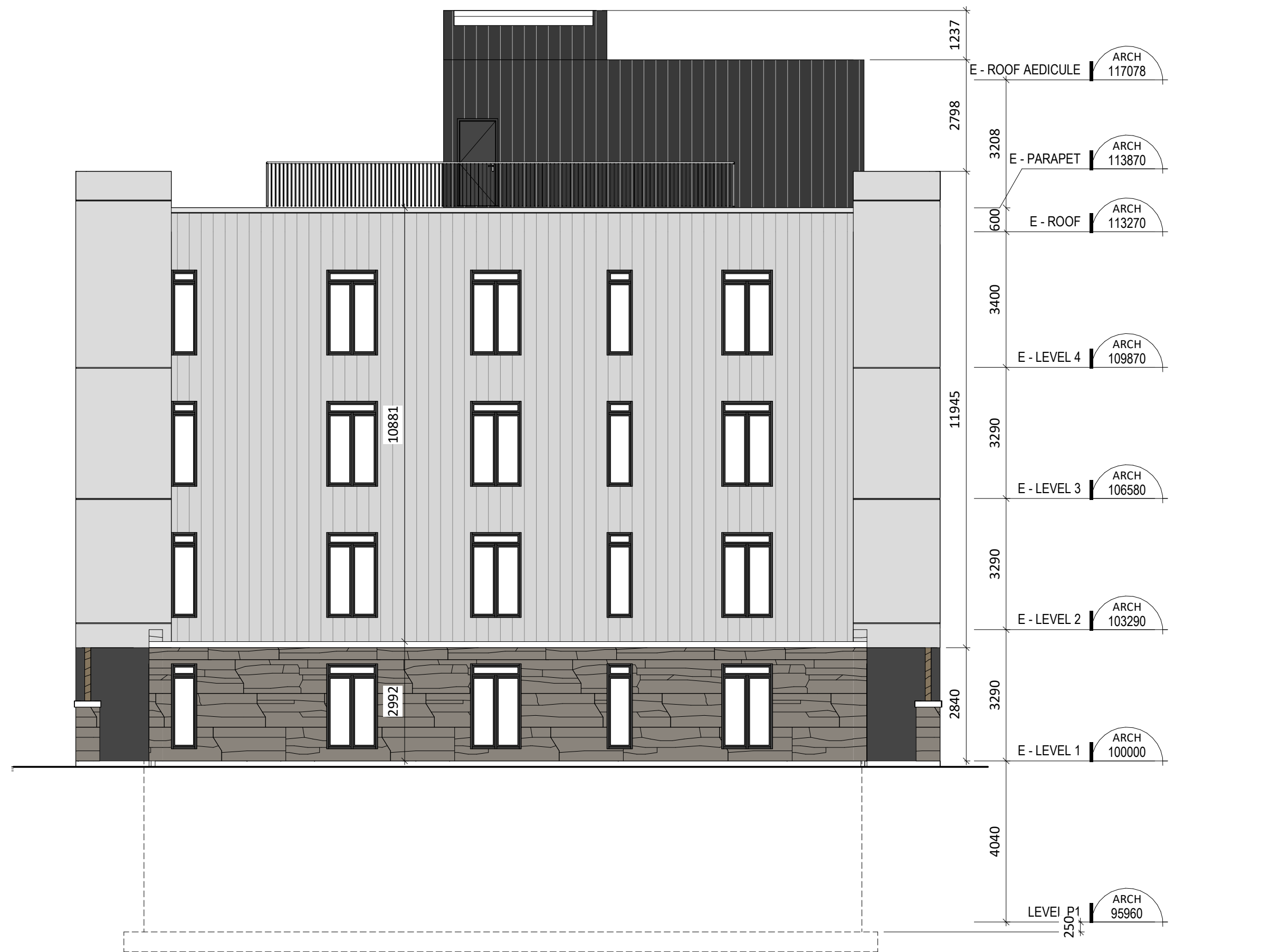
1 EAST ELEVATION - BUILDING E A301 1:100
