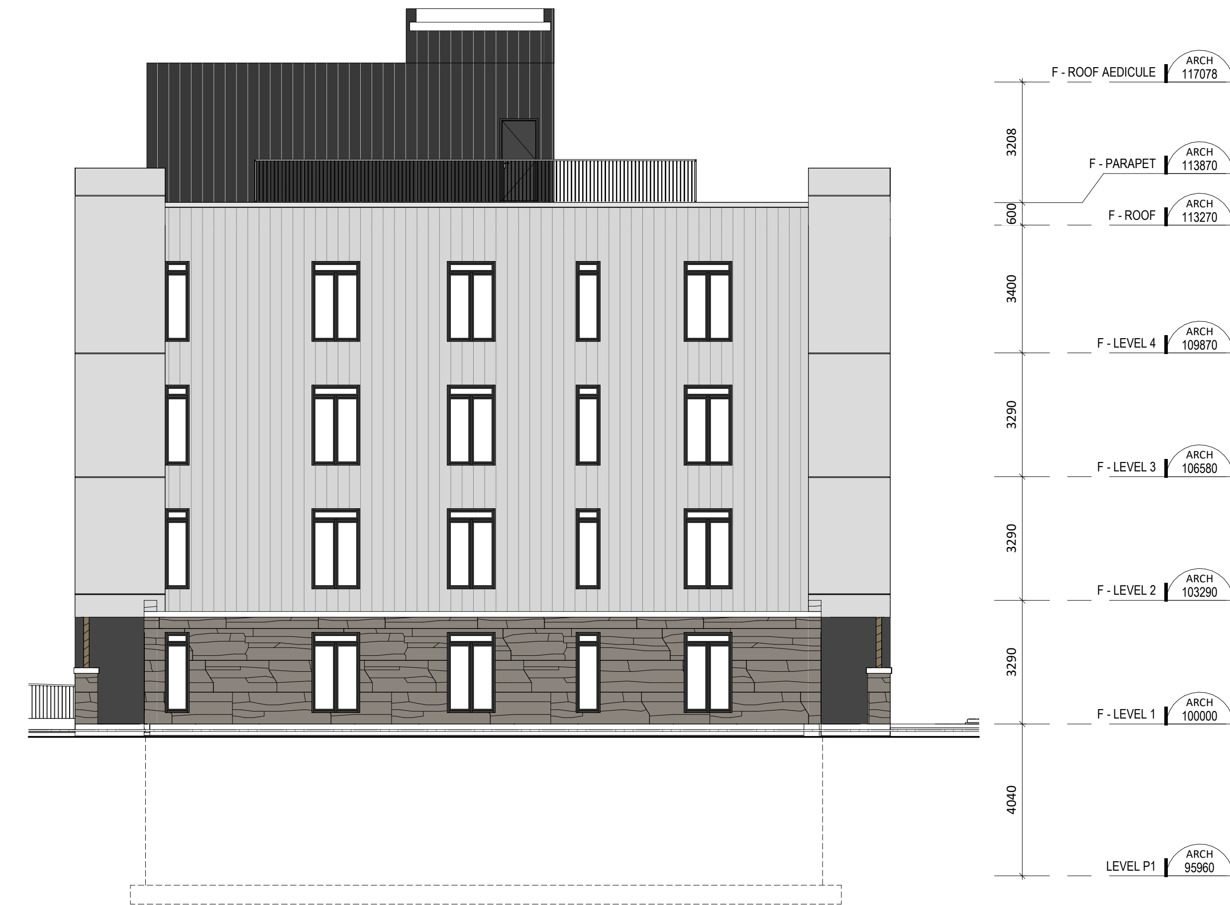
2 SOUTH ELEVATION - BUILDING F A302 1:100
