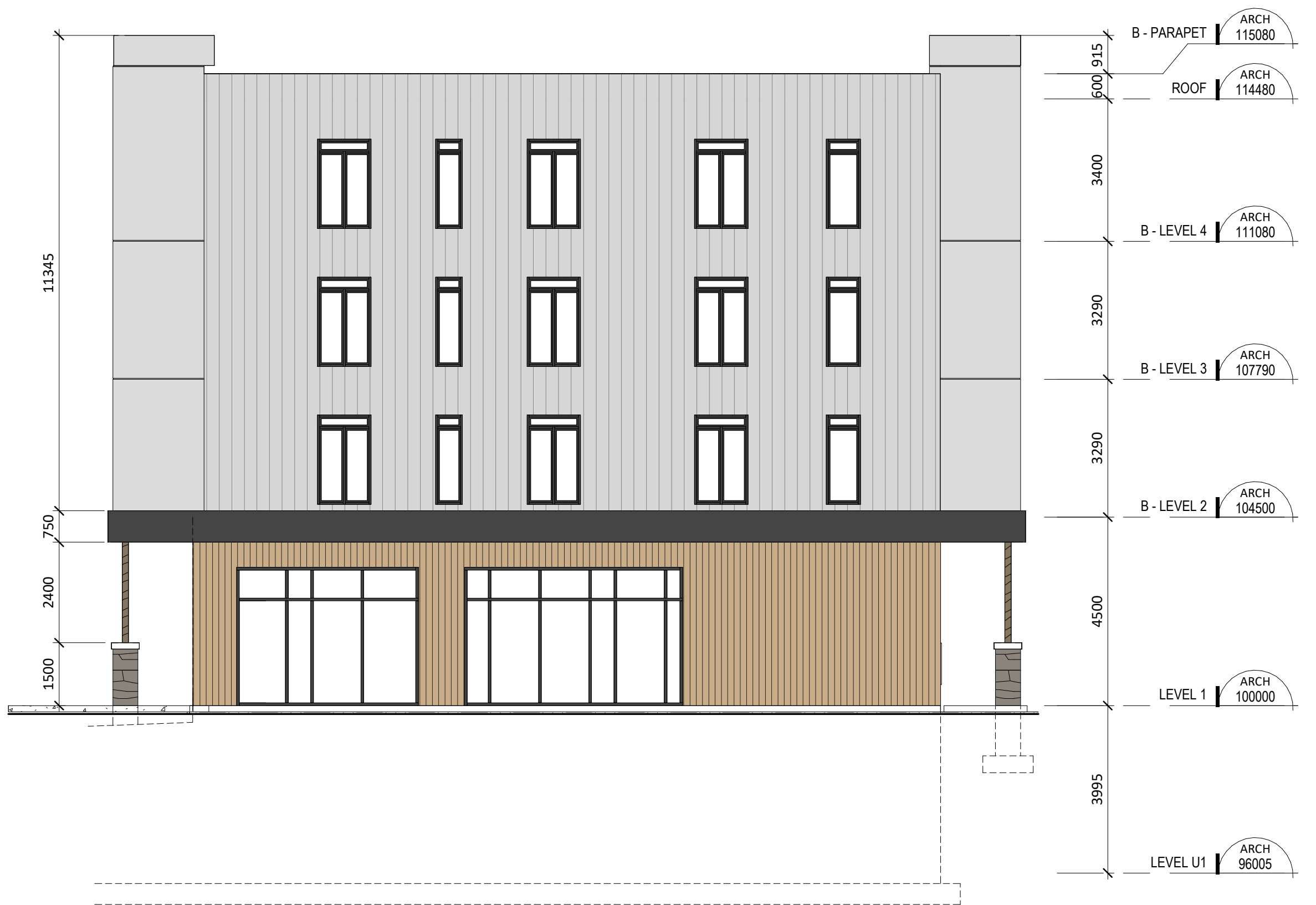
3 LEFT ELEVATION - BUILDING B A302 1 : 100
