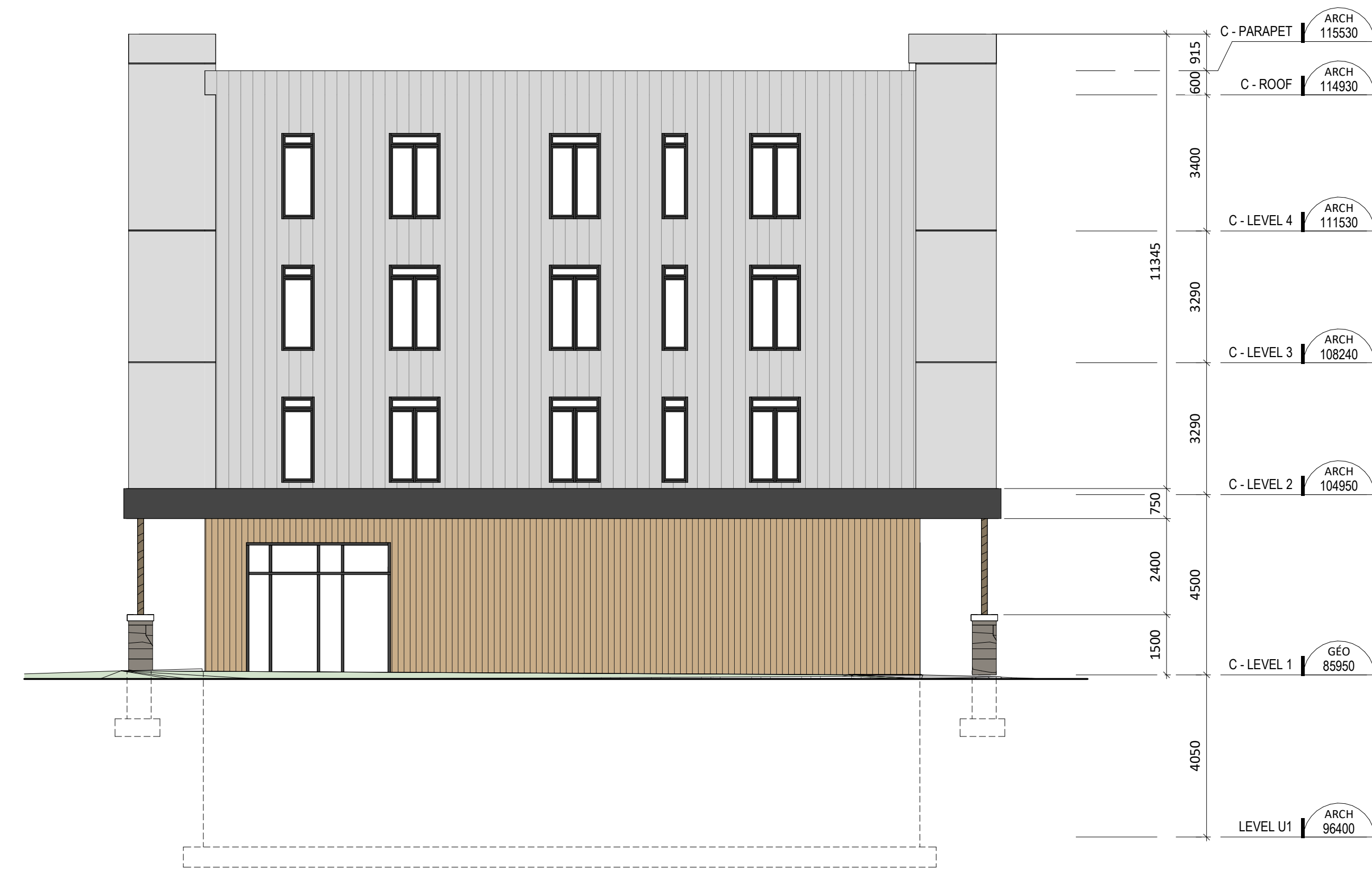
2 NORTH ELEVATION - BUILDING C A202 1:100
