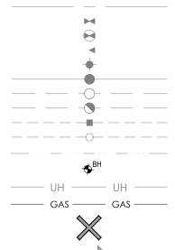
EXISTING WATERMAIN EXISTING VALVE AND VALVE BOX EXISTING VALVE CHAMBER EXISTING REDUCER EXISTING FIRE HYDRANT EXISTING SANITARY SEWER **EXISTING STORM SEWER** EXISTING CATCHBASIN MANHOLE **EXISTING CATCHBASIN** EXISTING SUBDRAIN CATCHBASIN EXISTING SWALE EXISTING BOREHOLE LOCATION EXISTING UNDERGROUND HYDRO EXISTING UNDERGROUND GAS
