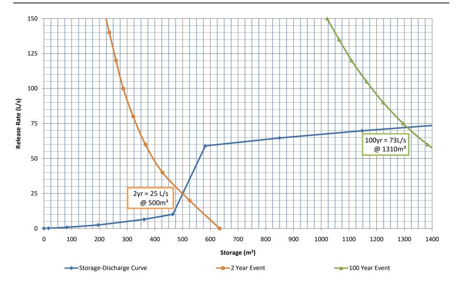
Figure 2: Stage-Storage Curve
